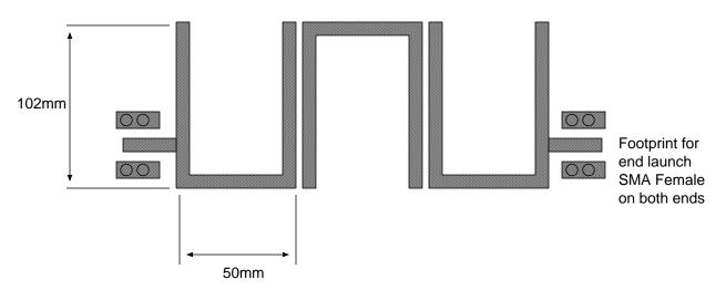
All resonators same dimensions Spacing between resonators is 0.5mm Line widths are 2.54mm Material: 0.062" FR4 with 2oz copper Full ground plan on bottom side ENIG
